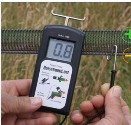
Touch "S" shaped wand to (-) line on Bipolar tape
