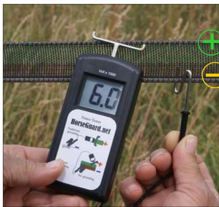
Touch "Y" shaped terminal to (+) line on Bipolar tape
